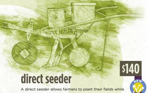
preserving the soil's fertility. The seeder has a cutting disk, ripper tine, and a slot that drops fertilizer and one seed at a time into the ground. Your gift of a direct seeder can help 3 to 5 farmers practice conservation agriculture methods to grow food.
